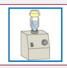
Vortex for mixing samples completely
